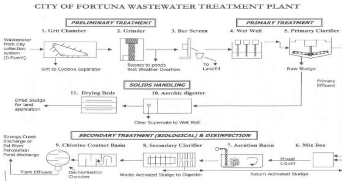
Figure 1 A schematic of the Fortuna wastewater treatment process, which describes the flow of wastewater through a network of biological, chemical and physical treatment processes.
